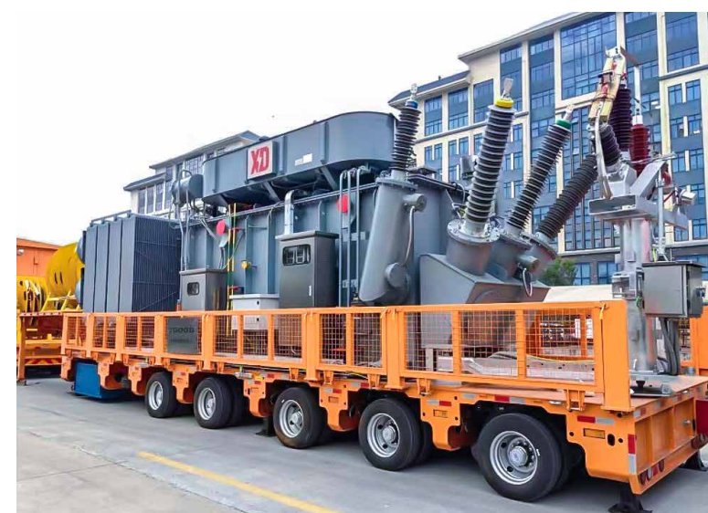
> Guangxi Hezhou 110 kV Mobile Trailer Substation
