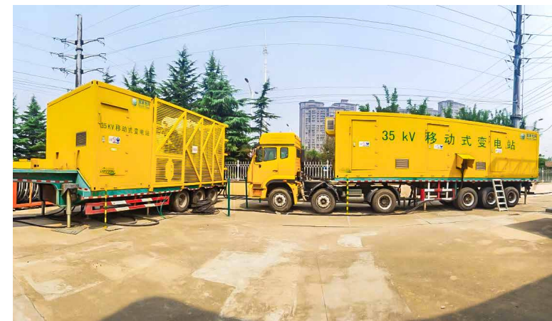
> Shandong Qingdao 35 kV Mobile Trailer Substation
