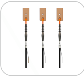
Rear View of Connection of Single Cable and Busbar in Switchgear
