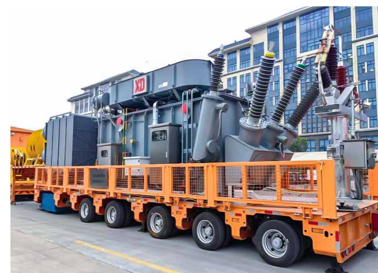
> Guangxi Hezhou 110 kV Mobile Trailer Substation
