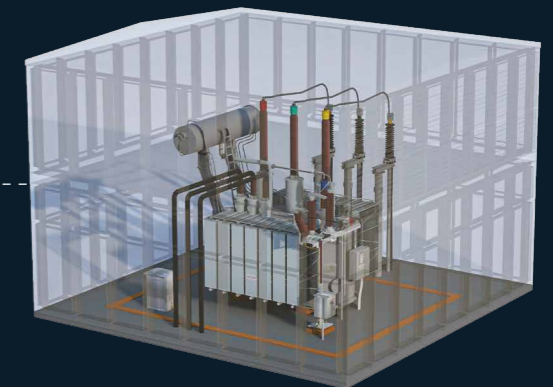
Integrated transformer compartment
