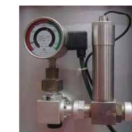
SF 6 gas online monitoring sensor
